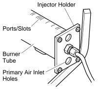
Figure 43 - Injector Holder On Outlet Burner Tube
